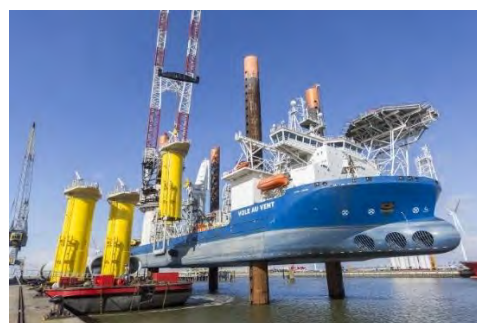
Figure 6-11: Foundation load-out using a jack-up vessel [63]
