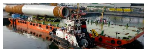
Figure 6-16: Roll-in / Roll-out Foundation transfer
