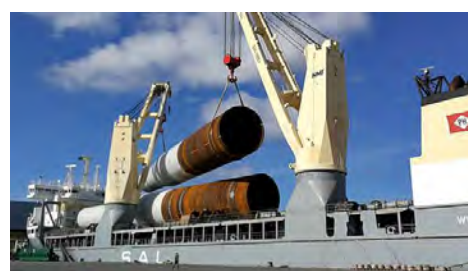
Figure 6-9: Transportation vessel with heavy lift cranes [61]
