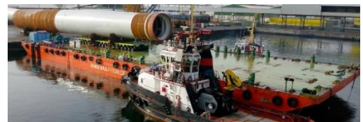
Figure 6-16: Roll-in/Roll-out Foundation transfer
